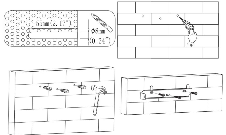
Fig 5.8 Schematic diagram of wall mount installation
