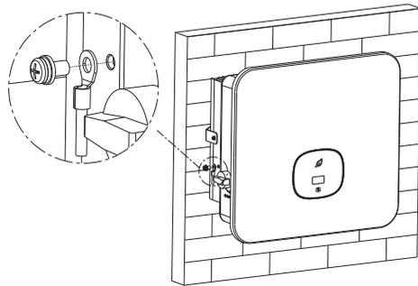
Fig 6.1 Grounding diagram
