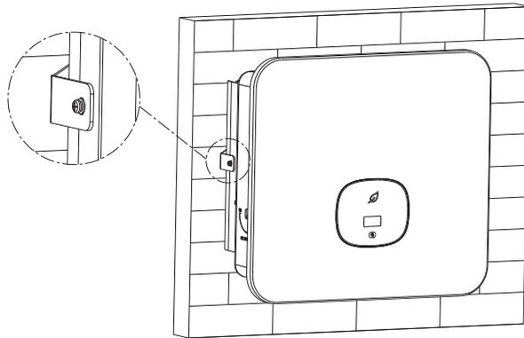
Fig 5.9 Schematic diagram of inverter wall mounting
